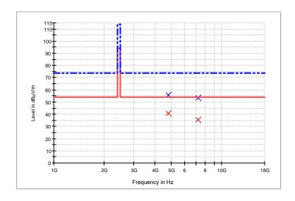
Note: Correction Factor = cable loss + antenna loss – preamp gain - receiver gain.
