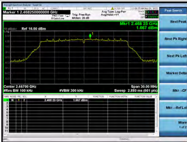
802.11n-20 MHz 12 CHANNEL, CARRIER LEVEL
