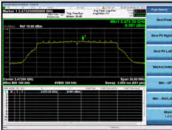
802.11n-20 MHz 13 CHANNEL, CARRIER LEVEL
