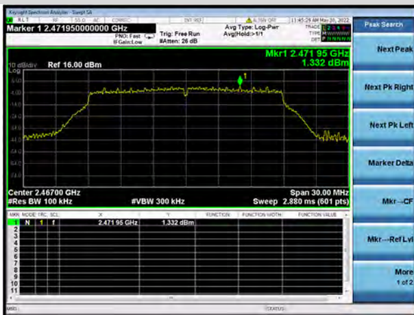
802.11n-20 MHz 12 CHANNEL, CARRIER LEVEL
