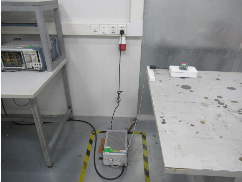
Photo of Conducted Emission Measurement
