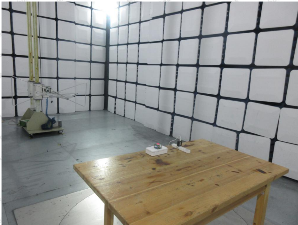
Photo of Radiation Emission Test
