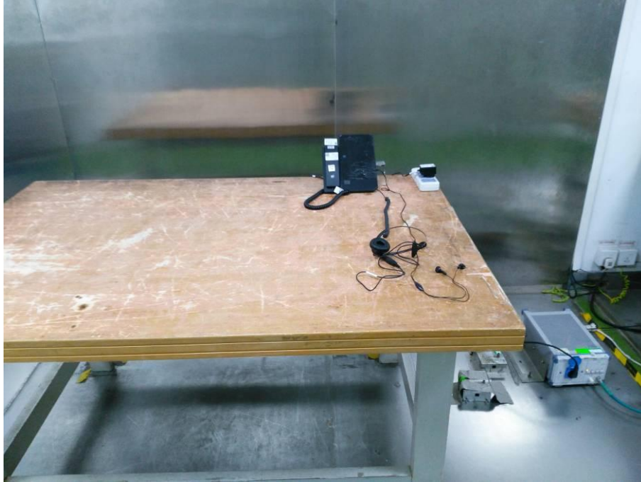
Conducted Emissions - Front View (Powered by adapter)
