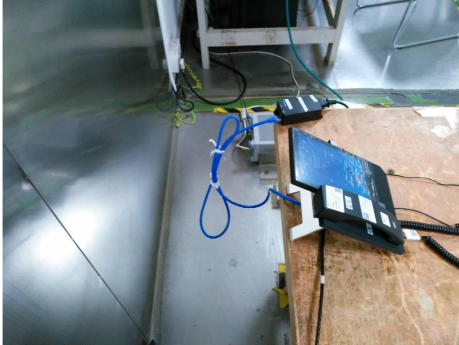
Conducted Emissions - Side View (Powered by POE)
