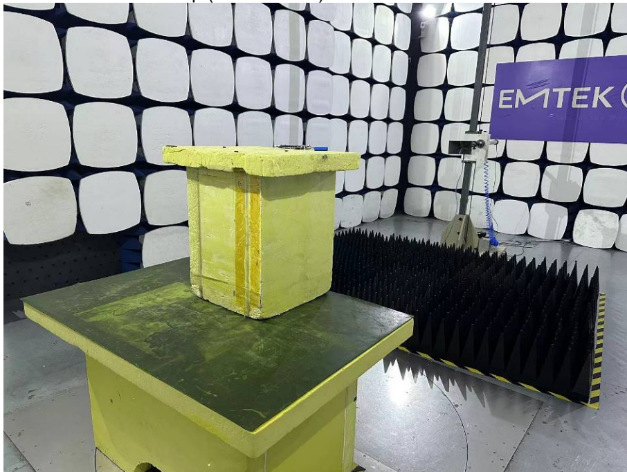
Spurious Emission Test Setup (Above 1GHz)
