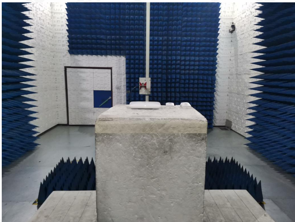
FCC RADIATED EMISSION TEST SETUP ABOVE 1GHZ
