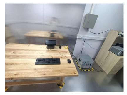
Radiated Emissions From 30MHz-1000MHz
