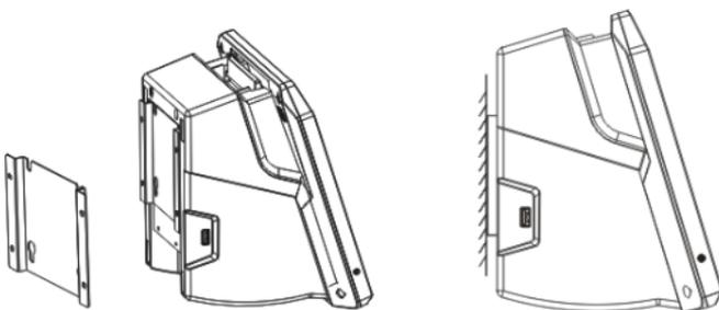
Step 1. A suitable flat wall should be required for installing fixture. Install the 4 screws that fixing the bracket on the wall, and install the 4 screws that embedding the equipment on the metal base board
