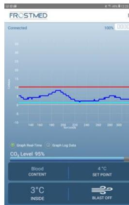
Figure 11: Blast function
