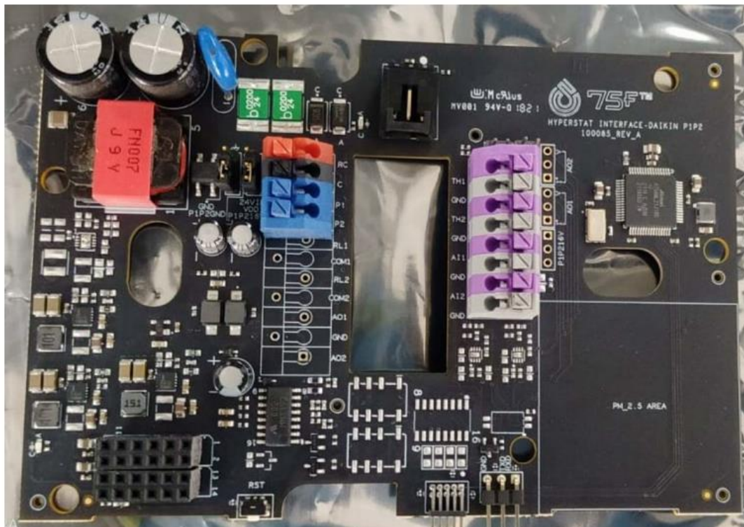
HyperStat Interface Daikin P1P2 Base PCB front view
