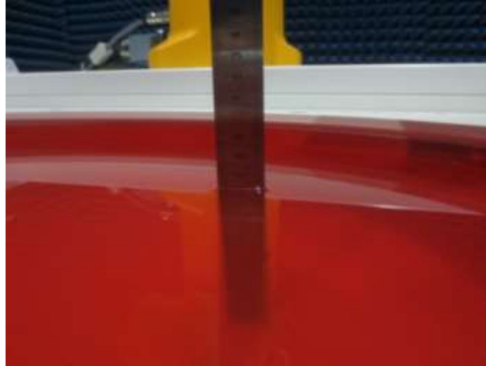
Fig. 9.6 Photo of Liquid Height for Body SAR of ELI V5.0 (5000MHz~5800MHz) (depth>15cm)
