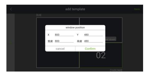
(6) When the parameters of the position and size of this 3 windows are set, click "save" in the upper right corner to complete the custom template operation, and it will automatically return to adding template interface, and then you will be able to see the newly added 1600x960 multi window template, as shown below:
