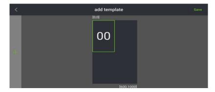
(2) In the 00 box, press your finger slightly on the edge of the frame and slide it in the direction you want to drag. Slide your finger to drag the frame so that the green frame is drawn to the widest and highest state, i.e.: fill 600x1000, as following figure shows:
