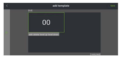
(4) Slightly press the "00" which inside the 00 window frame with your finger, s when the bottom edge of the box appears: edit, delete, move up, move down, click "edit" to set the position and size of the 00 window, enter the X, Y, Width, Height of the 00 window, as shown below:
