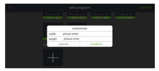
(2) For example: respectively input 1600 and 960 for width and height, click "OK" to jump to the adding templates interface, as shown in the figure below:
