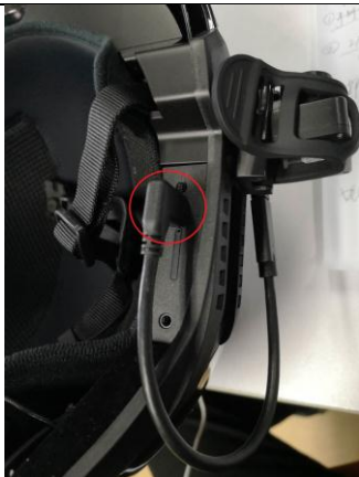
Figure 5. Connection of thermal imaging module
