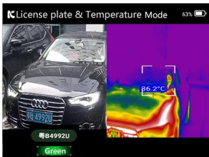
Figure 26. License plate recognition & temperature measurement mode
