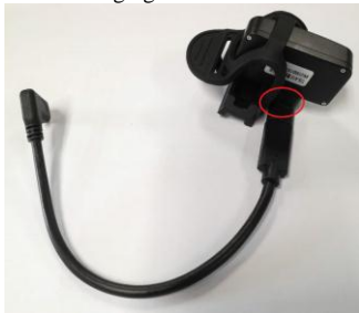
Figure 3. Connect thermal imaging module to connector
