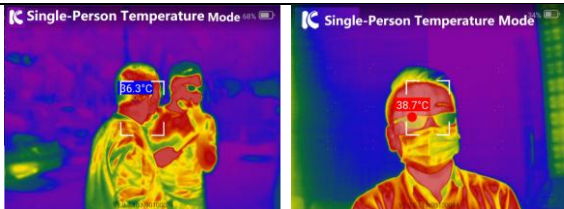
Figure 21. Single-person temperature measurement mode
