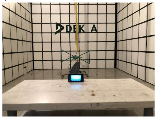
Description: Radiated Emission Test Setup for 1~18GHz
