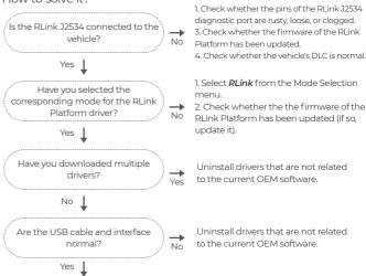
Check whether the USB cable is damaged, aged, flattened, or the interface is corroded. Check whether the computer USB interface is normal, or try again with another
