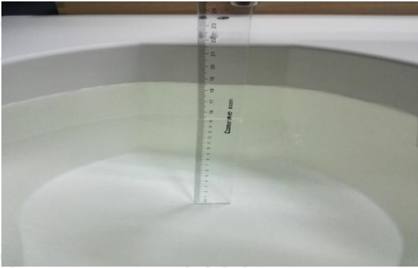
The Body Liquid of 2450MHz (15.3cm)
