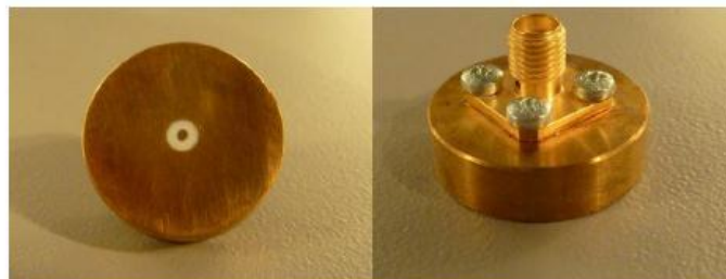
Figure 1 – MVG LIMESAR Dielectric Probe
