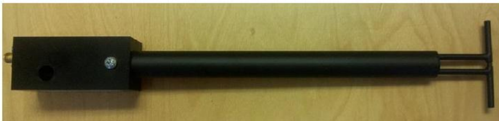
Figure 1 – MVG COMOSAR Validation Dipole
