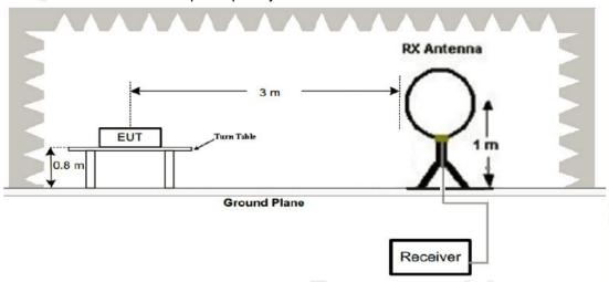
2. Radiated Emission Test-Up Frequency 30MHz~1GHz
