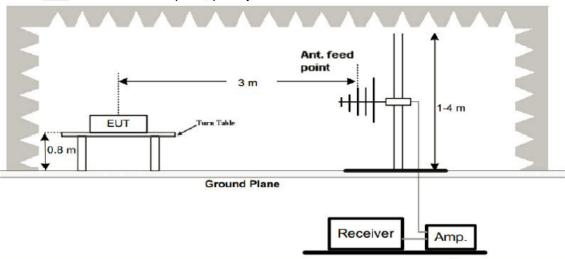
3. Radiated Emission Test-Up Frequency Above 1GHz
