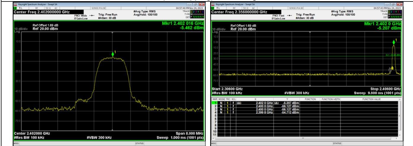
$\pi/4$ -DQPSK(No-Hopping): Band Edge, Right Side
