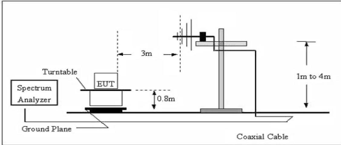
Radiated emission test-up frequency above 1GHz
