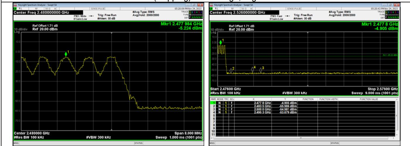
$\pi/4$ -DQPSK(Hopping): Band Edge, Left Side
