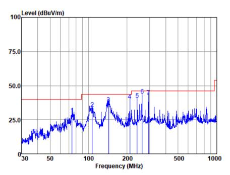
Antenna Polarity : HORIZONTAL EUT/Project :1807CR
