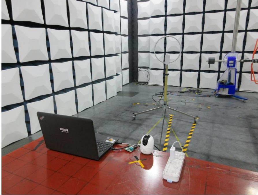
RADIATED RF MEASUREMENT SETUP (9KHz ~ 30 MHz)
