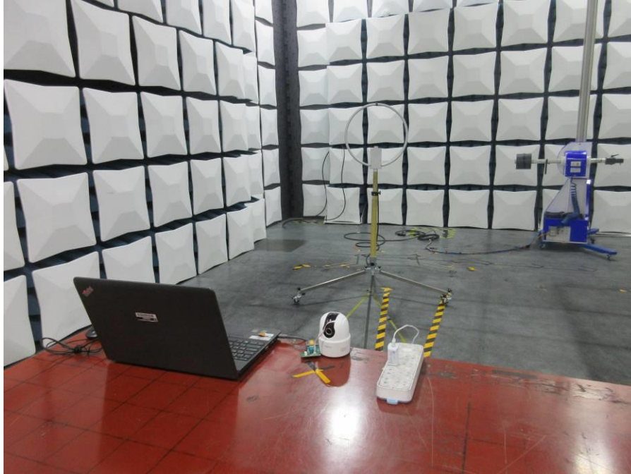
RADIATED RF MEASUREMENT SETUP (9KHz ~ 30 MHz)
