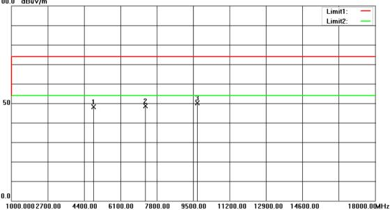
No. Frequency Reading Correct Result Limit Margin Remark (MHz) (dBuV) Factor(dB/m) (dBuV/m) (dBuV/m) (dB) 4844.000 58.24 74.00 1 -10.1348.11 -25.89peak 2 7266.000 55.65 -7.00 48.65 74.00 -25.35 peak 3 9688.000 54.76 -4.58 50.18 74.00 -23.82 peak
