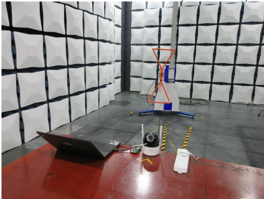
RADIATED RF MEASUREMENT SETUP (30MHz ~ 1 GHz)
