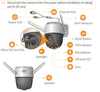
Press and hold the reset button for 10 s to reset the camera. • Double-press the reset button to enable camera's hotspot.
