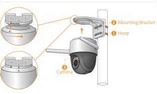
attach the bracket to the pole .
