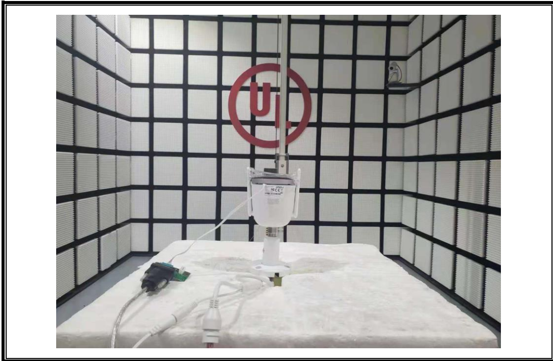
RADIATED RF MEASUREMENT SETUP (Above 1G – Y axis)
