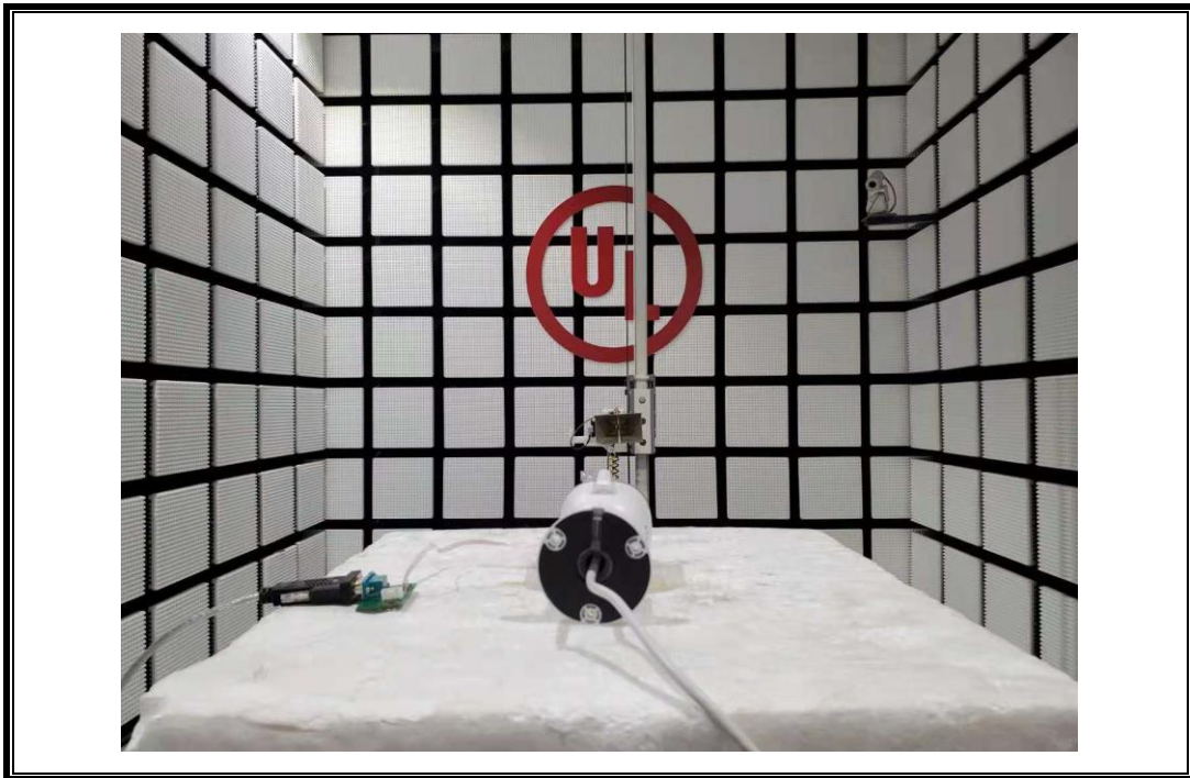
RADIATED RF MEASUREMENT SETUP (Above 1G – Y axis)
