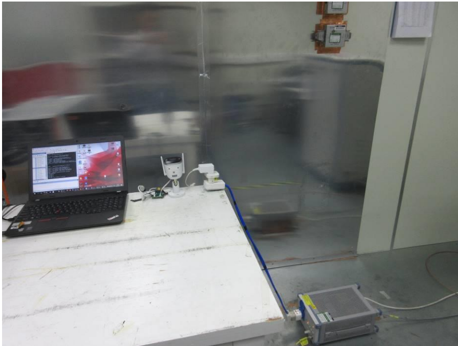
POWERLINE CONDUCTED EMISSIONS MEASUREMENT SETUP
