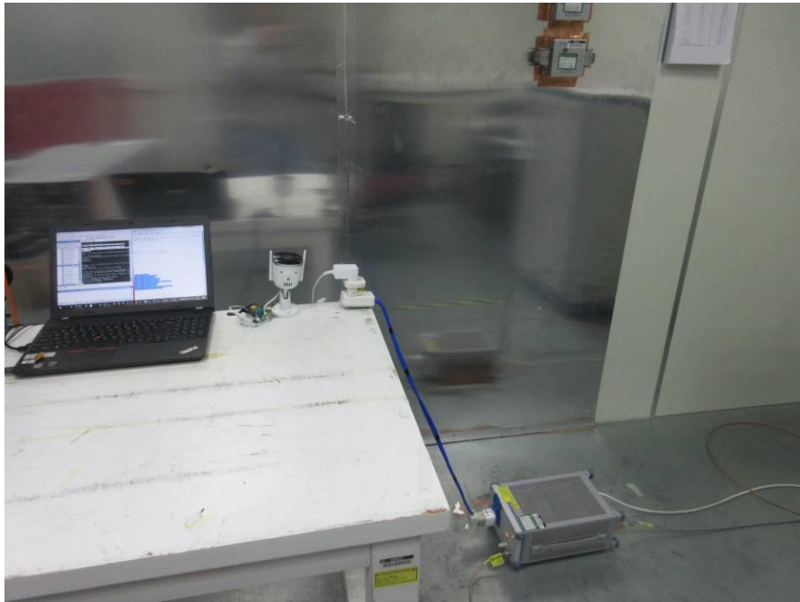
POWERLINE CONDUCTED EMISSIONS MEASUREMENT SETUP
