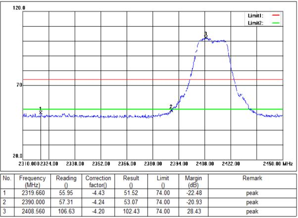
Mode:a; Polarization:Horizontal; Modulation:g; bandwidth:20MHz; Channel:Low
