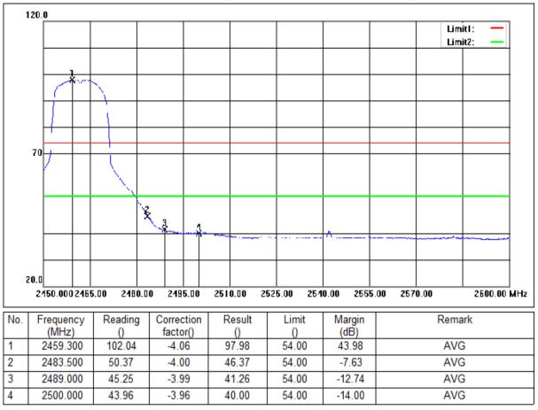
Mode:a; Polarization:Vertical; Modulation:g; bandwidth:20MHz; Channel:High
