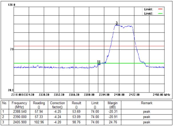
Mode:a; Polarization:Horizontal; Modulation:n; bandwidth:20MHz; Channel:Low
