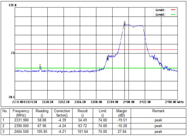
Mode:a; Polarization:Vertical; Modulation:n; bandwidth:20MHz; Channel:Low
