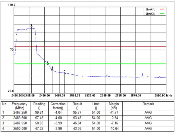
Mode:a; Polarization:Vertical; Modulation:n; bandwidth:20MHz; Channel:High
