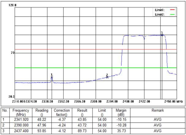
Mode:a; Polarization:Vertical; Modulation:n; bandwidth:40MHz; Channel:Low
