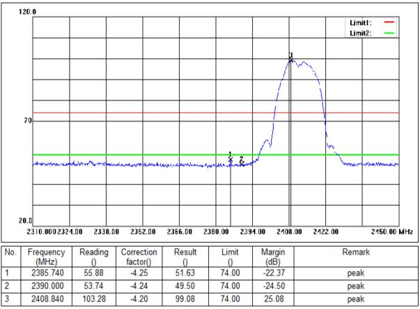
Mode:a; Polarization:Horizontal; Modulation:b; bandwidth:20MHz; Channel:Low
