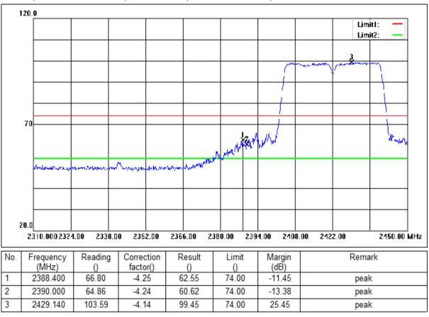
Mode:a; Polarization:Vertical; Modulation:n; bandwidth:40MHz; Channel:Low
