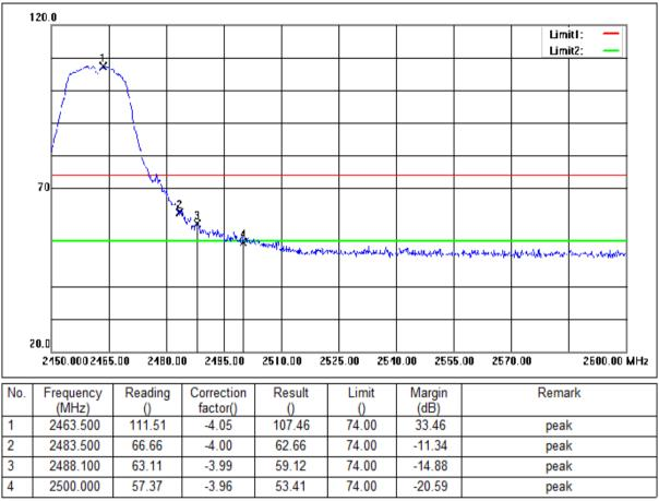
Mode:a; Polarization:Vertical; Modulation:g; bandwidth:20MHz; Channel:High
