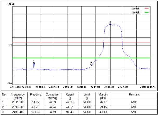
Mode:a; Polarization:Vertical; Modulation:g; bandwidth:20MHz; Channel:Low
