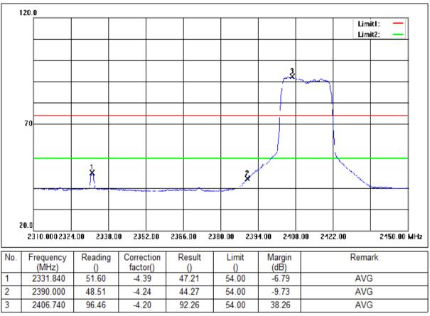
Mode:a; Polarization:Vertical; Modulation:n; bandwidth:20MHz; Channel:Low
