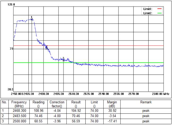
Mode:a; Polarization:Vertical; Modulation:n; bandwidth:20MHz; Channel:High
