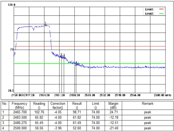
Mode:a; Polarization:Vertical; Modulation:n; bandwidth:40MHz; Channel:High
