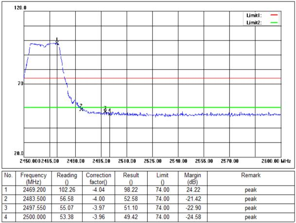
Mode:a; Polarization:Horizontal; Modulation:n; bandwidth:20MHz; Channel:High
