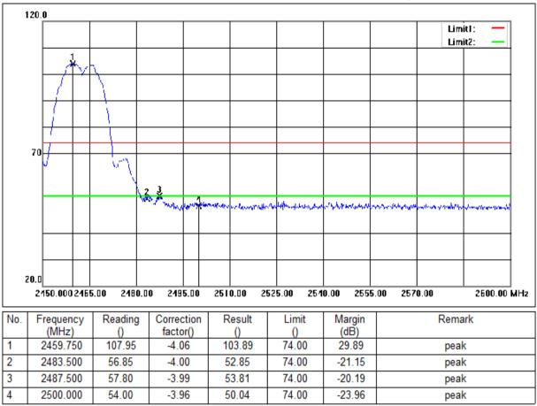
Mode:a; Polarization:Vertical; Modulation:b; bandwidth:20MHz; Channel:High
