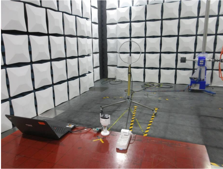
RADIATED RF MEASUREMENT SETUP (9KHz ~ 30 MHz)
