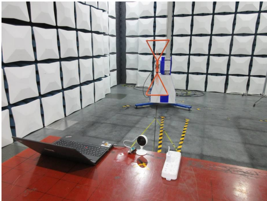
RADIATED RF MEASUREMENT SETUP (30MHz ~ 1 GHz)
