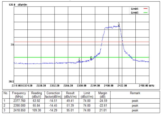
Mode:a; Polarization:Vertical; Modulation:g; bandwidth:20MHz; Channel:Low
