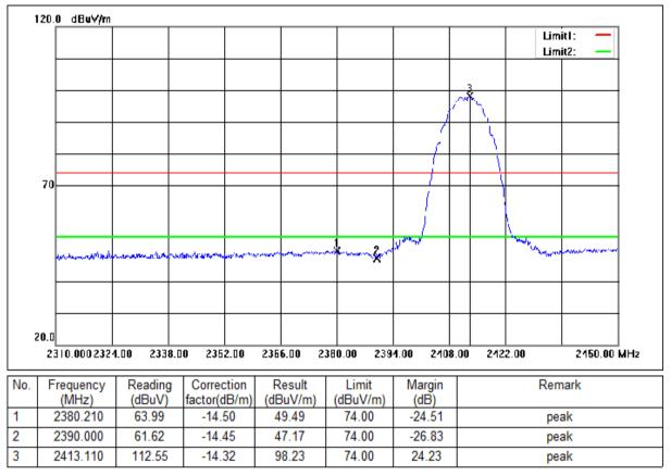
Mode:a; Polarization:Vertical; Modulation:b; bandwidth:20MHz; Channel:Low
