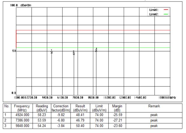
Mode:a; Polarization:Horizontal; Modulation:n; bandwidth:20MHz; Channel:High
