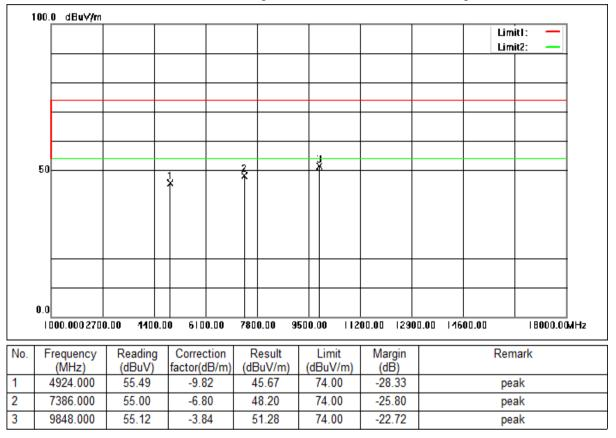
Mode:a; Polarization:Vertical; Modulation:g; bandwidth:20MHz; Channel:High
