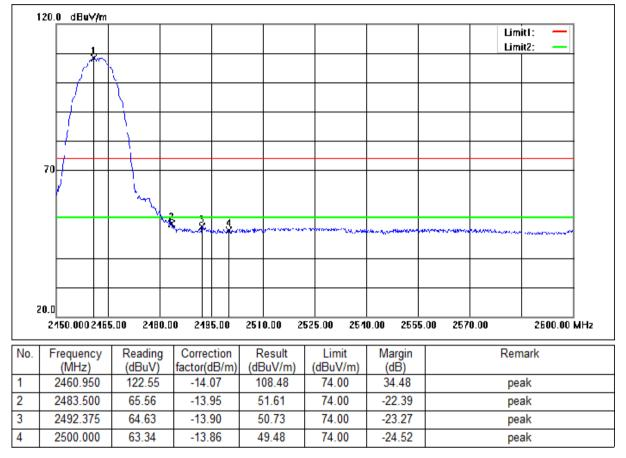
Mode:a; Polarization:Horizontal; Modulation:b; bandwidth:20MHz; Channel:High
