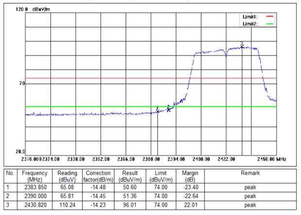
Mode:a; Polarization:Vertical; Modulation:n; bandwidth:40MHz; Channel:Low
