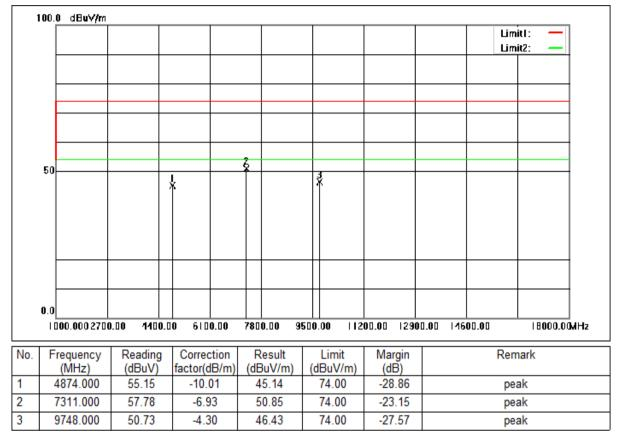
Mode:a; Polarization:Horizontal; Modulation:b; bandwidth:20MHz; Channel:middle
