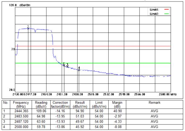
Mode:a; Polarization:Horizontal; Modulation:n; bandwidth:40MHz; Channel:High
