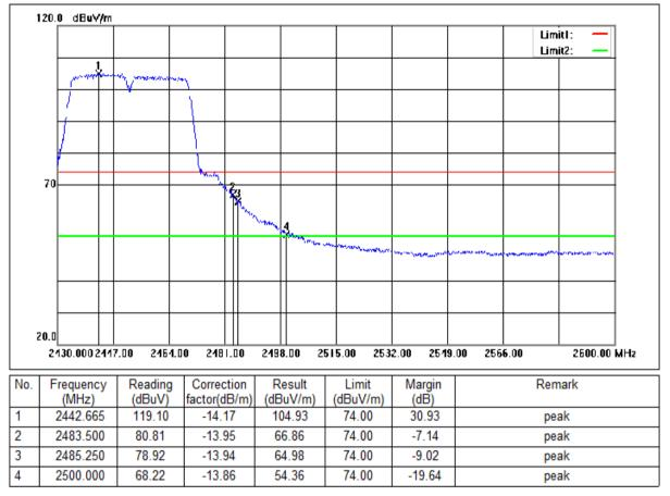
Mode:a; Polarization:Horizontal; Modulation:n; bandwidth:40MHz; Channel:High
