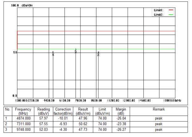
Mode:a; Polarization:Vertical; Modulation:n; bandwidth:40MHz; Channel:middle
