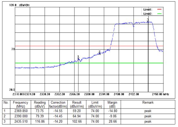
Mode:a; Polarization:Horizontal; Modulation:n; bandwidth:40MHz; Channel:Low
