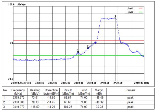
Mode:a; Polarization:Horizontal; Modulation:n; bandwidth:20MHz; Channel:Low
