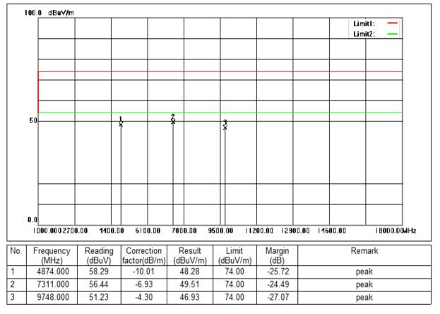
Mode:a; Polarization:Vertical; Modulation:b; bandwidth:20MHz; Channel:middle
