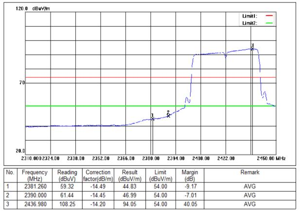
Mode:a; Polarization:Horizontal; Modulation:n; bandwidth:40MHz; Channel:Low
