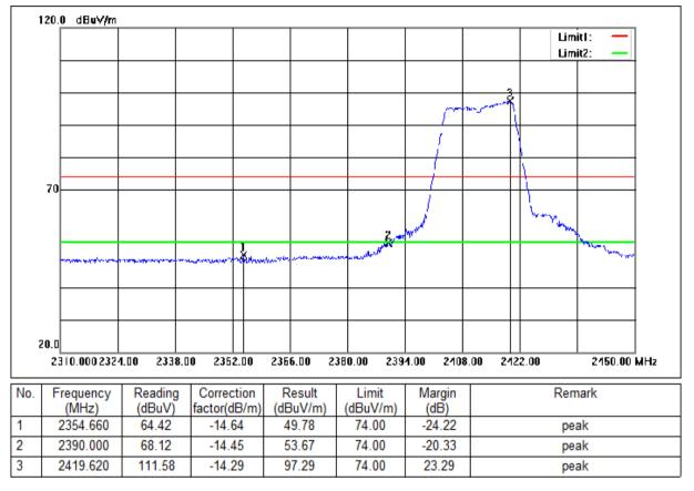
Mode:a; Polarization:Vertical; Modulation:n; bandwidth:20MHz; Channel:Low
