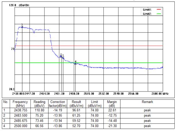
Mode:a; Polarization:Vertical; Modulation:n; bandwidth:40MHz; Channel:High
