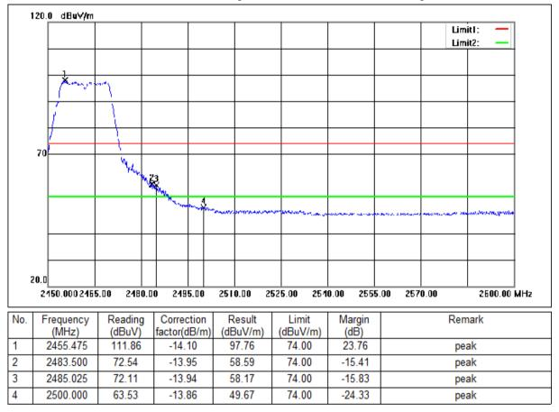
Mode:a; Polarization:Vertical; Modulation:g; bandwidth:20MHz; Channel:High
