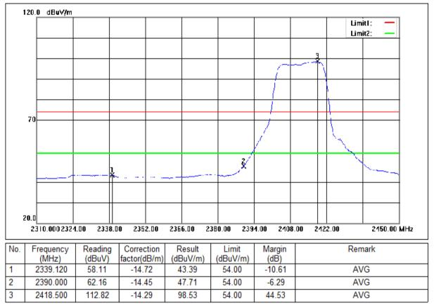
Mode:a; Polarization:Horizontal; Modulation:n; bandwidth:20MHz; Channel:Low
