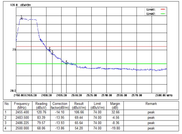
Mode:a; Polarization:Horizontal; Modulation:n; bandwidth:20MHz; Channel:High
