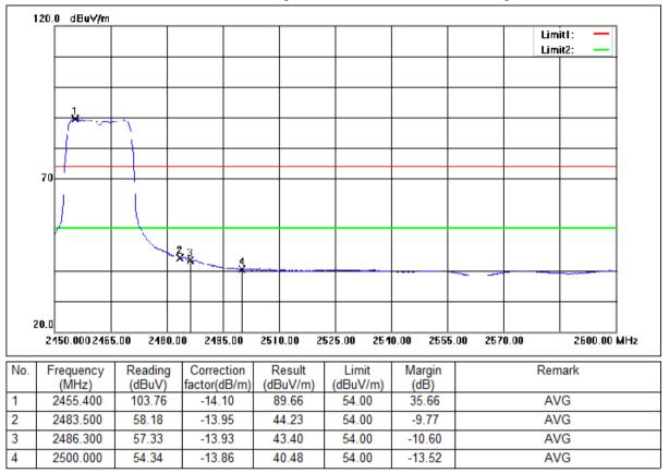
Mode:a; Polarization:Vertical; Modulation:g; bandwidth:20MHz; Channel:High
