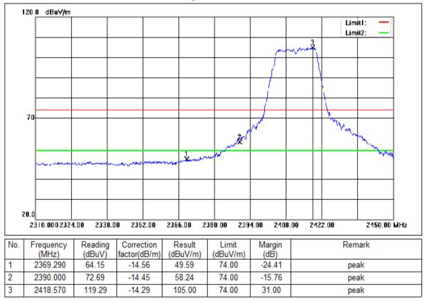
Mode:a; Polarization:Horizontal; Modulation:g; bandwidth:20MHz; Channel:Low
