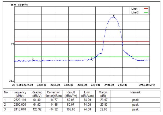
Mode:a; Polarization:Horizontal; Modulation:b; bandwidth:20MHz; Channel:Low
