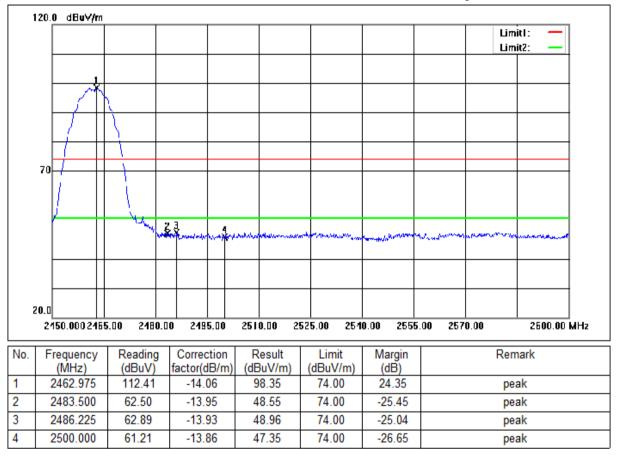
Mode:a; Polarization:Vertical; Modulation:b; bandwidth:20MHz; Channel:High
