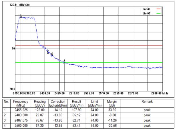
Mode:a; Polarization:Horizontal; Modulation:g; bandwidth:20MHz; Channel:High
