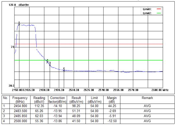
Mode:a; Polarization:Horizontal; Modulation:n; bandwidth:20MHz; Channel:High
