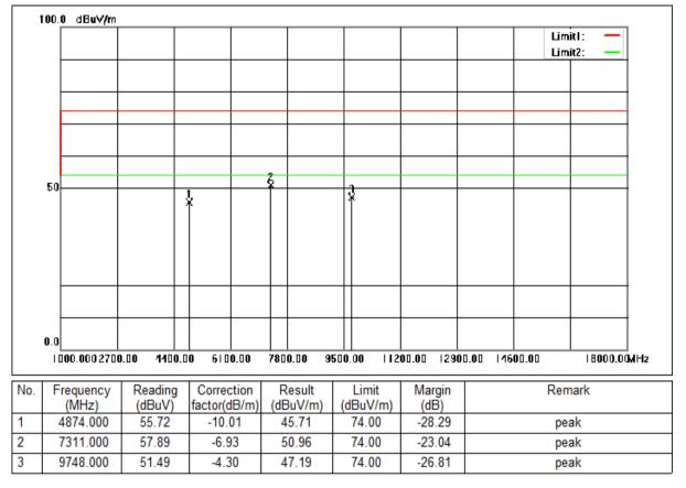
Mode:a; Polarization:Horizontal; Modulation:n; bandwidth:20MHz; Channel:middle
