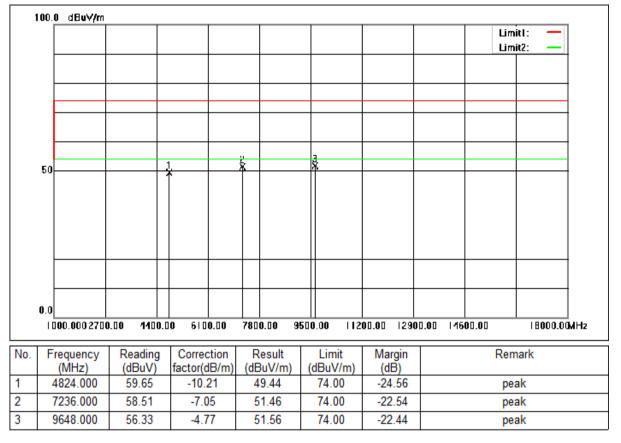
Mode:a; Polarization:Vertical; Modulation:n; bandwidth:20MHz; Channel:Low
