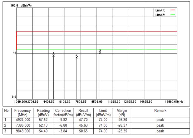
Mode:a; Polarization:Vertical; Modulation:b; bandwidth:20MHz; Channel:High
