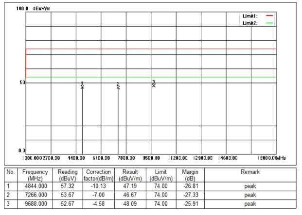
Mode:a; Polarization:Vertical; Modulation:n; bandwidth:40MHz; Channel:Low
