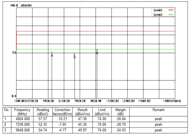
Mode:a; Polarization:Vertical; Modulation:g; bandwidth:20MHz; Channel:Low
