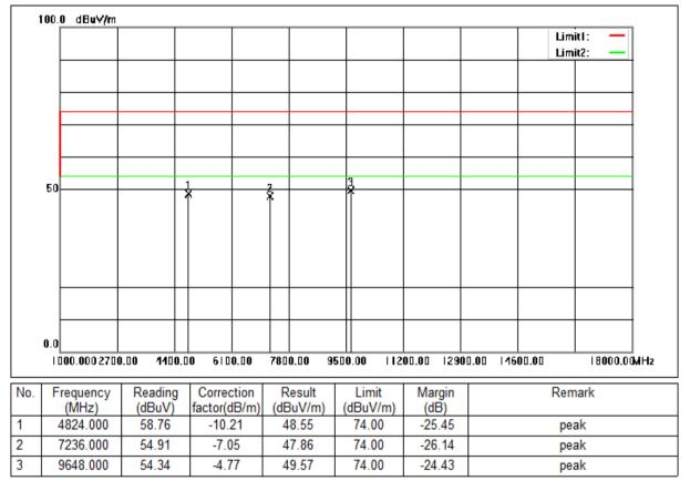
Mode:a; Polarization:Vertical; Modulation:b; bandwidth:20MHz; Channel:Low
