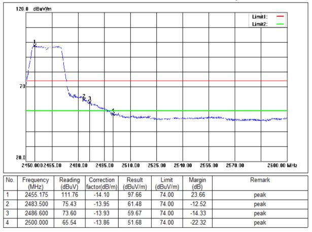
Mode:a; Polarization:Vertical; Modulation:n; bandwidth:20MHz; Channel:High
