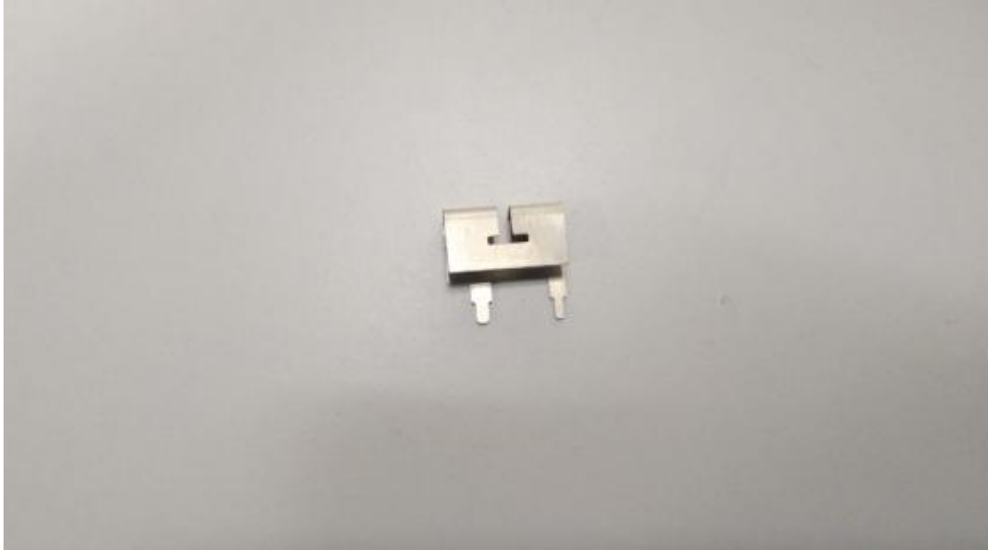
Figure 1 0337 (A12 Project) WIFI Antenna
