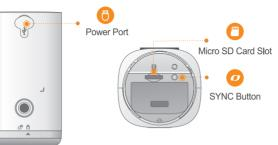
Note: Press the SYNC button to pair with the base station. Press and hold the SYNC button until you hear beep sound.
