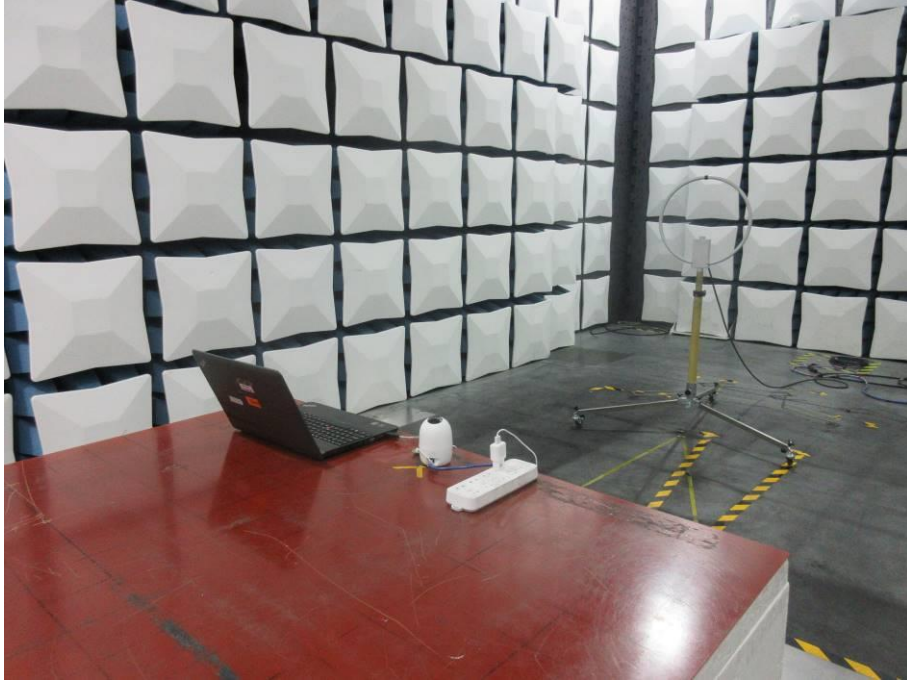
RADIATED RF MEASUREMENT SETUP (9KHz ~ 30 MHz)
