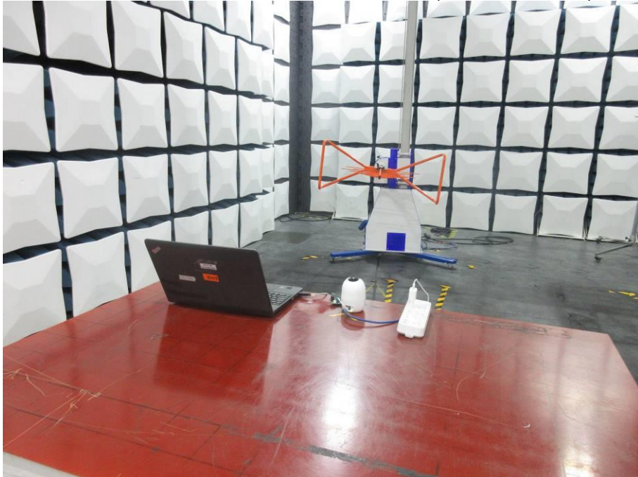
RADIATED RF MEASUREMENT SETUP (30MHz ~ 1 GHz)
