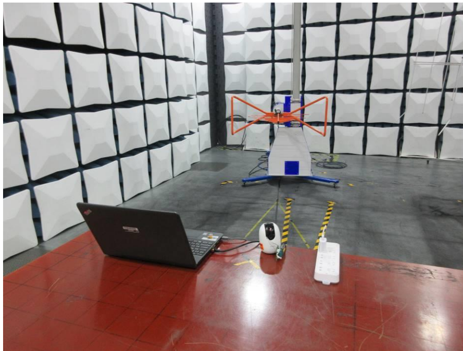
RADIATED RF MEASUREMENT SETUP (30MHz ~ 1 GHz)
