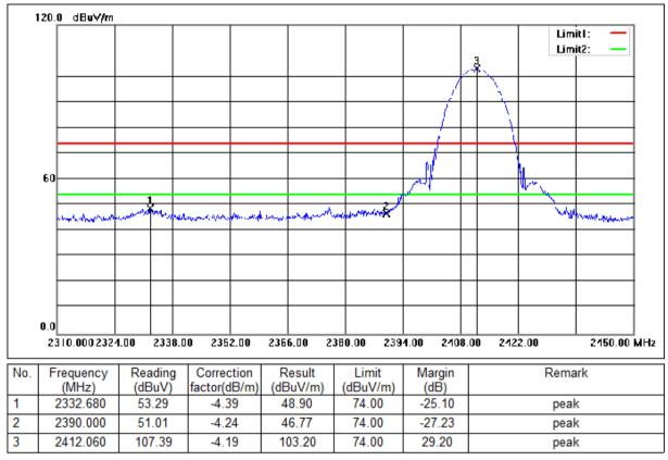
Mode:a; Polarization:Vertical; Modulation:b; bandwidth:20MHz; Channel:Low
