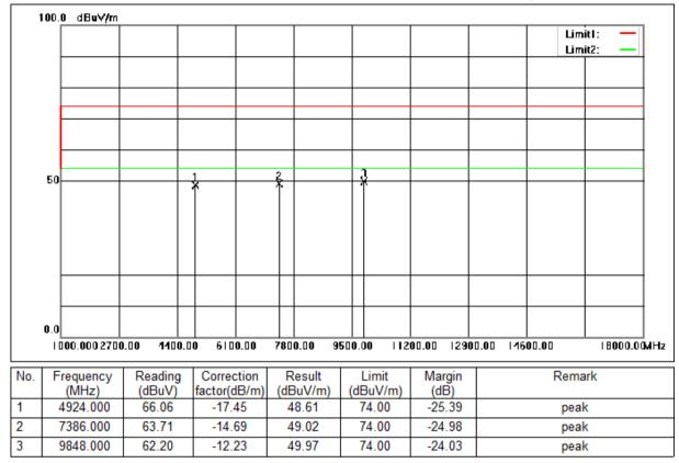
Mode:a; Polarization:Horizontal; Modulation:n; bandwidth:20MHz; Channel:High
