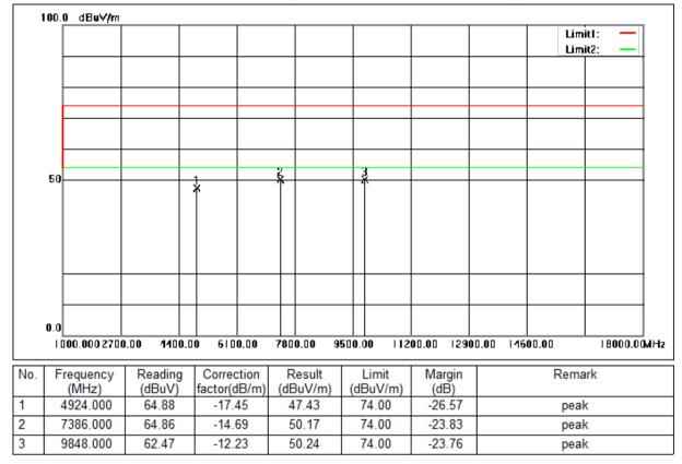
Mode:a; Polarization:Vertical; Modulation:g; bandwidth:20MHz; Channel:High
