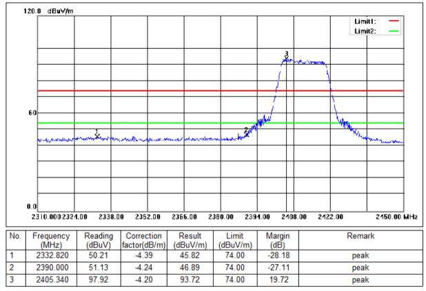
Mode:a; Polarization:Horizontal; Modulation:n; bandwidth:20MHz; Channel:Low
