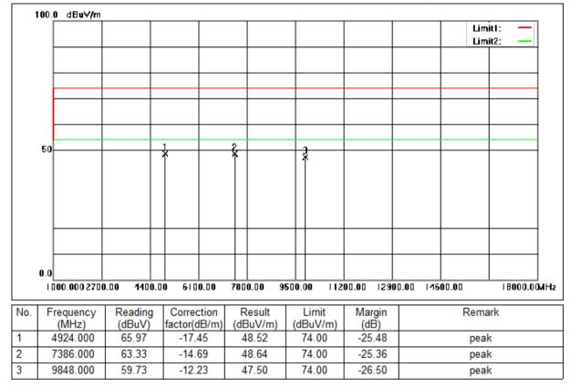
Mode:a; Polarization:Vertical; Modulation:b; bandwidth:20MHz; Channel:High
