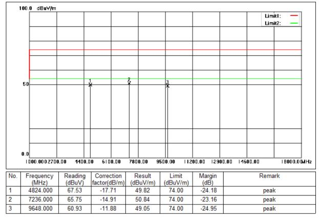
Mode:a; Polarization:Vertical; Modulation:b; bandwidth:20MHz; Channel:Low
