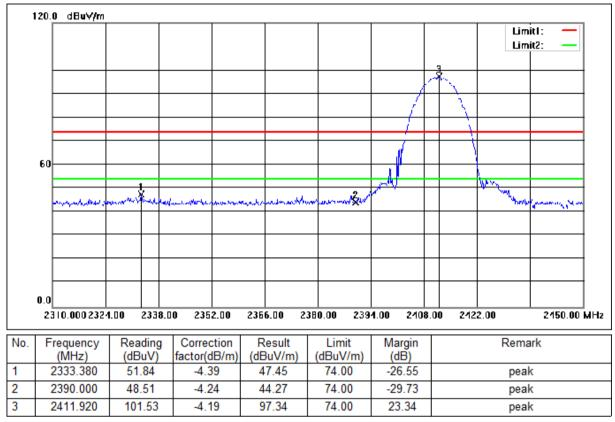
Mode:a; Polarization:Horizontal; Modulation:b; bandwidth:20MHz; Channel:Low
