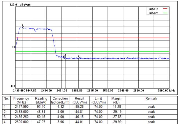
Mode:a; Polarization:Horizontal; Modulation:n; bandwidth:40MHz; Channel:High
