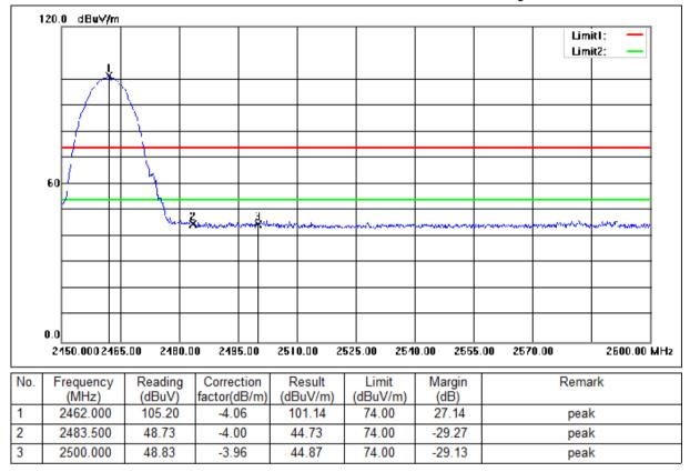
Mode:a; Polarization:Vertical; Modulation:b; bandwidth:20MHz; Channel:High
