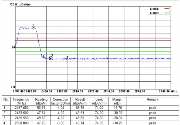
Mode:a; Polarization:Horizontal; Modulation:g; bandwidth:20MHz; Channel:High
