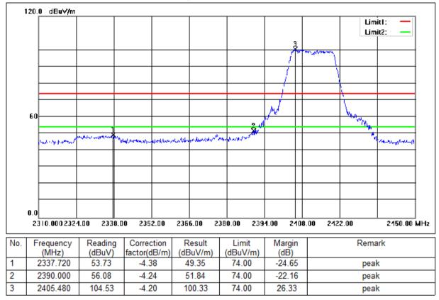
Mode:a; Polarization:Vertical; Modulation:g; bandwidth:20MHz; Channel:Low
