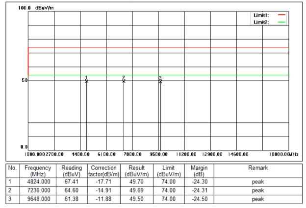
Mode:a; Polarization:Vertical; Modulation:g; bandwidth:20MHz; Channel:Low
