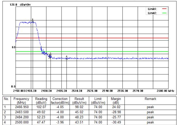
Mode:a; Polarization:Vertical; Modulation:g; bandwidth:20MHz; Channel:High
