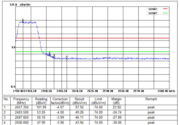
Mode:a; Polarization:Vertical; Modulation:n; bandwidth:20MHz; Channel:High
