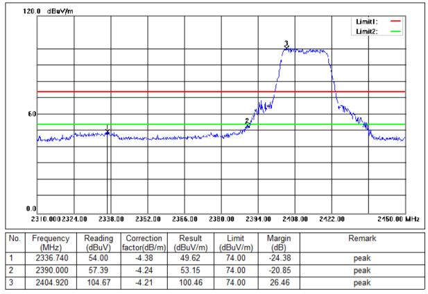
Mode:a; Polarization:Vertical; Modulation:n; bandwidth:20MHz; Channel:Low
