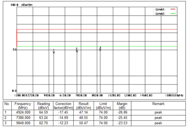
Mode:a; Polarization:Horizontal; Modulation:g; bandwidth:20MHz; Channel:High
