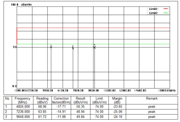
Mode:a; Polarization:Vertical; Modulation:n; bandwidth:20MHz; Channel:Low
