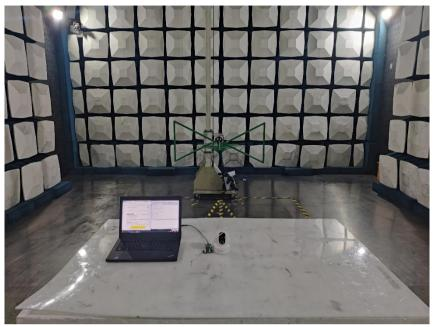
**Radiated Test Above 1GHz**
