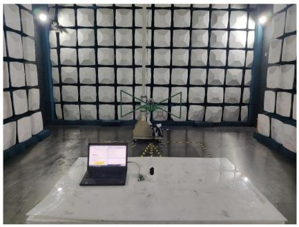
**Radiated Test Above 1GHz**
