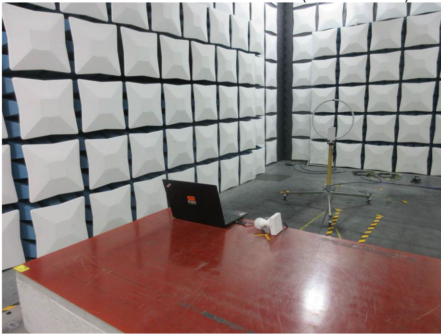
RADIATED RF MEASUREMENT SETUP (9kHz ~ 30 MHz)
