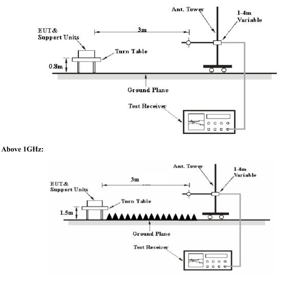
The radiated emissions were performed in the 3 meters distance, using the setup accordance with the ANSI C63.10-2013. The specification used was the FCC 15.209 and FCC 15.249, RSS-Gen limits.
