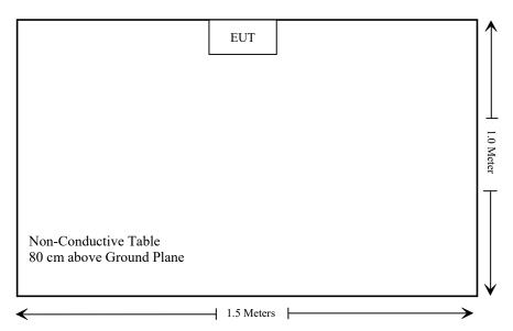
Note: the support table edge was flush with the center of turntable
