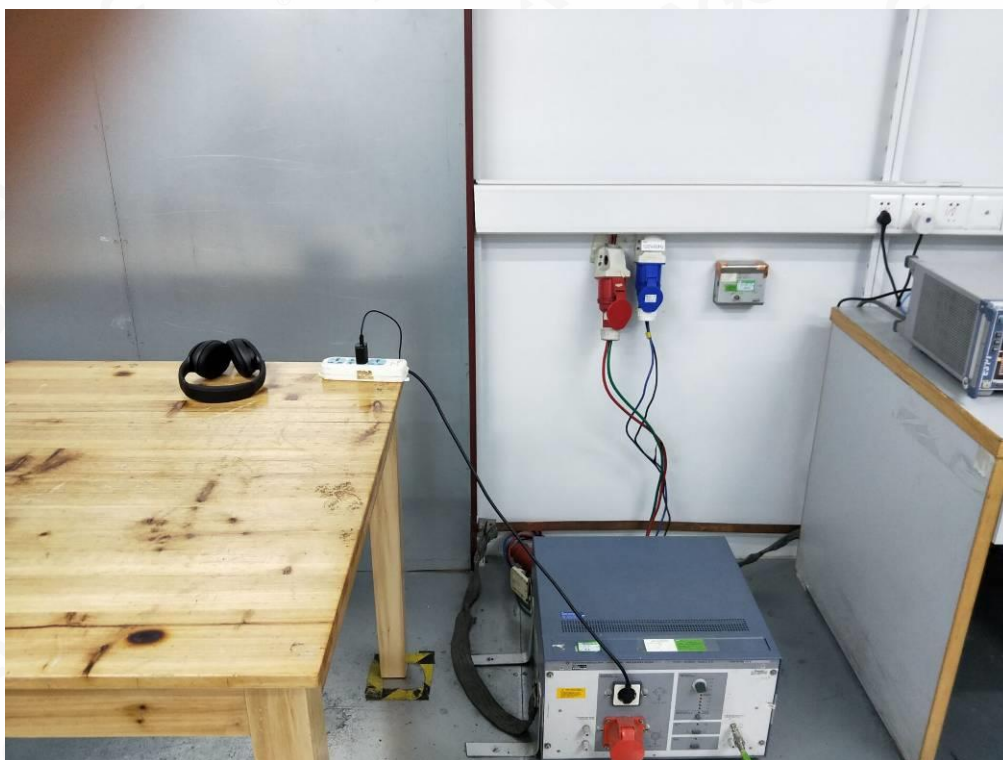
RADIATED EMISSION TEST SETUP BELOW 1GHZ
