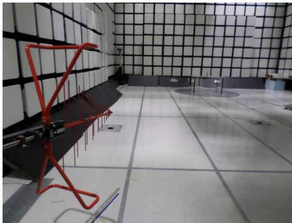
Figure 4: Remote Control - RSE - 30-1000 MHz - Setup Antenna View
