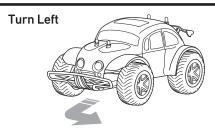
Push the throttle lever forwards and press the steering lever to the left.
