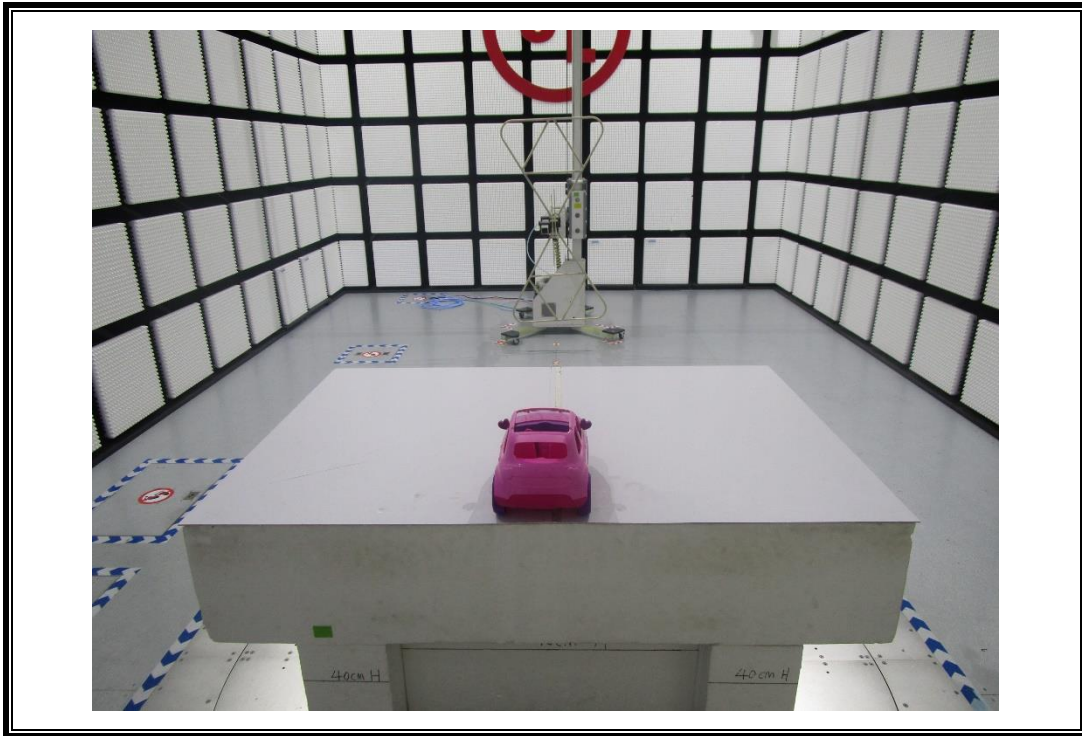
RADIATED RF MEASUREMENT SETUP (30MHz ~ 1 GHz)
