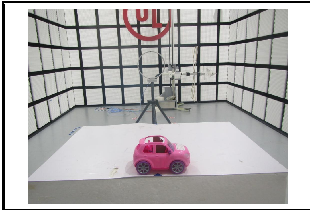
RADIATED RF MEASUREMENT SETUP (Below 30MHz)
