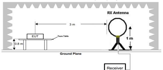
2. Radiated Emission Test Set-Up, Frequency below 1000MHz
