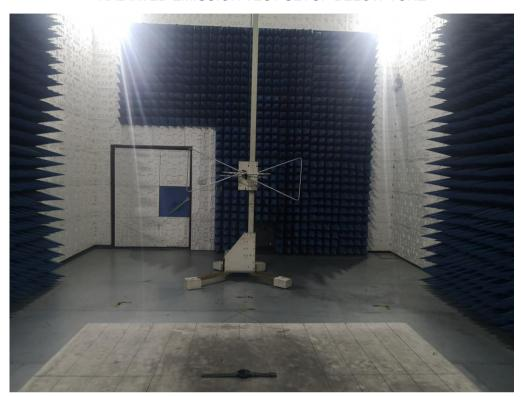
RADIATED EMISSION TEST SETUP ABOVE 1GHZ
