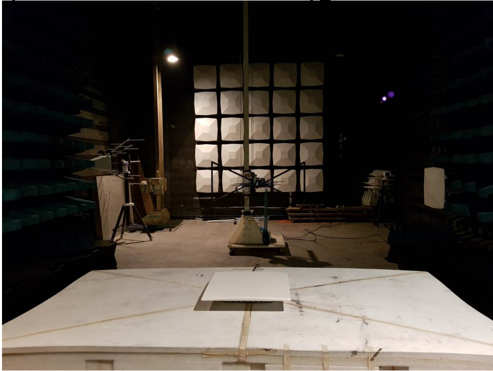
Photograph – Radiated Emission Test Set up Below 1GHz
